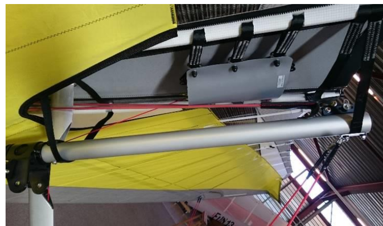
Figure 5-2 : Path of Tensioning Cables
